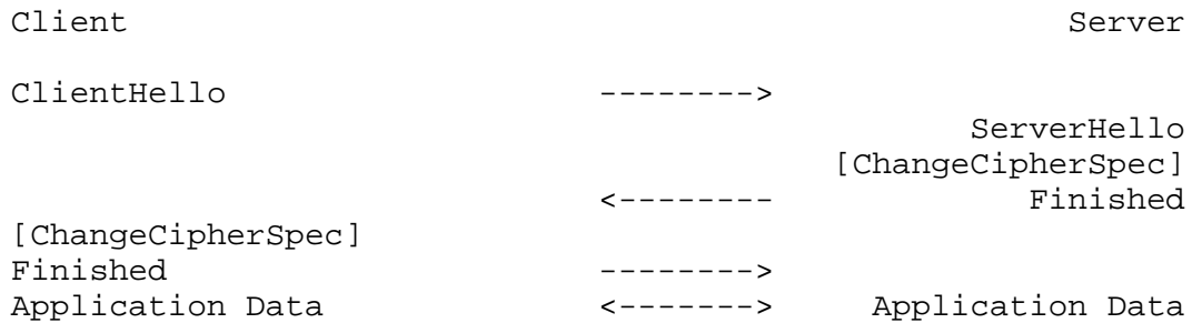
Figure 2. Message flow for an abbreviated handshake
